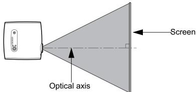
A slight error in the projection angle can be corrected using the KEYSTONE button. (P31)
